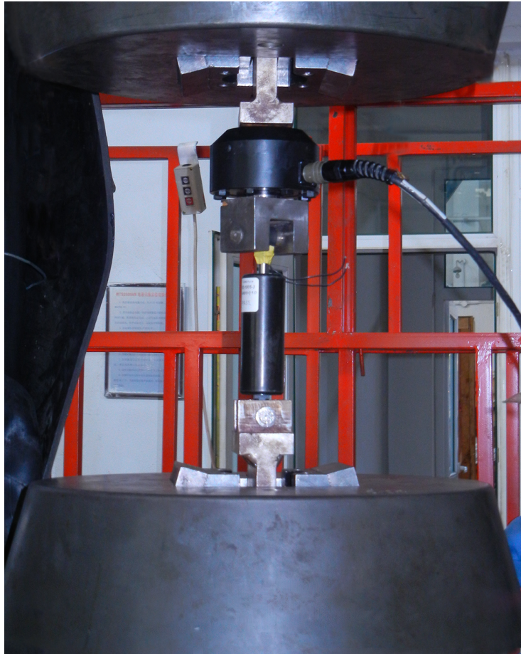
Figure 2.24: MTS Loading Frame with MR damper and Load Cell attached at HIT
