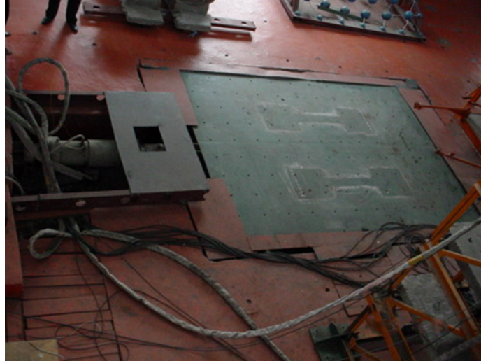
Figure 2.8: Shake table located at HIT
